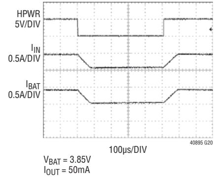
**Wall Connect Waveforms**
