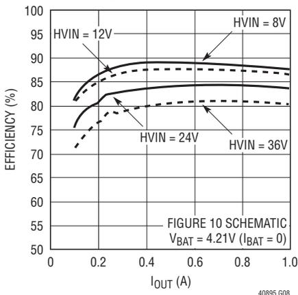
**LTC4089-5 High Voltage Regulator Efficiency vs Output Load**
