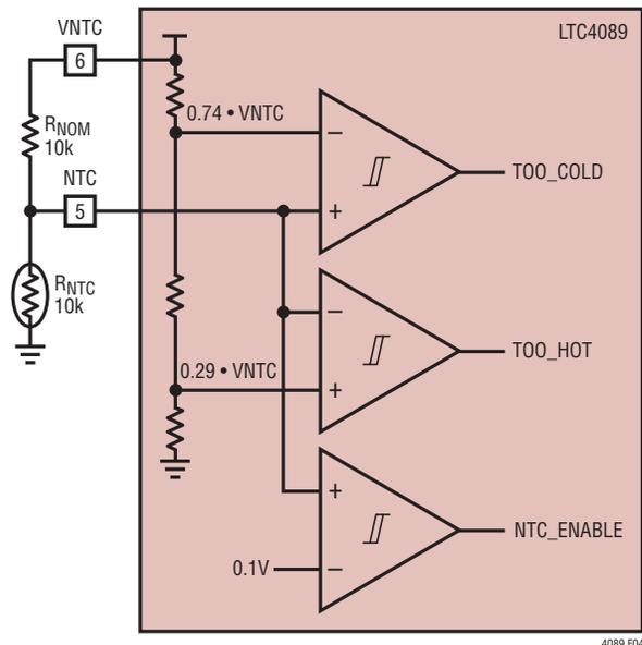
Figure 4. NTC Circuit
