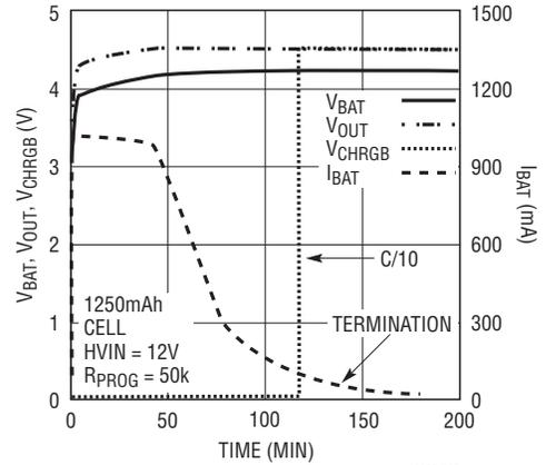
**Charging from USB, I<sub>BAT</sub> vs V<sub>BAT</sub>**
