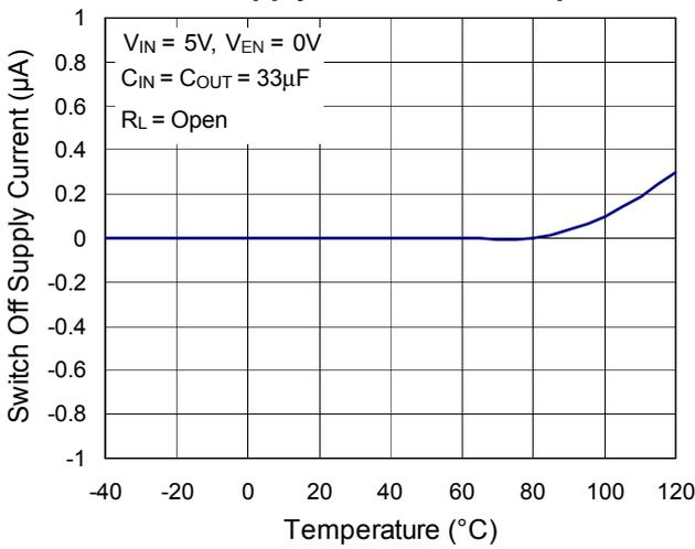
Turn-Off Leakage Current vs. Temperature ②
