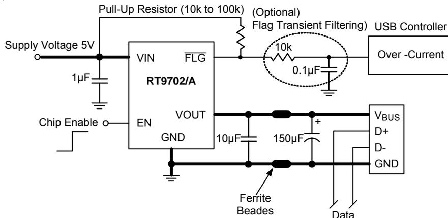
**Note:** A low-ESR 150µF aluminum electrolytic or tantalum between V<sub>OUT</sub> and GND is strongly recommended to meet the 330mV maximum droop requirement in the hub V<sub>BUS</sub>. (see Application Information Section for further details)
