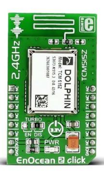
**EnOcean 2 click** carries the TCM 515Z transceiver, based on the **2.4 GHz** IEEE 802.15.4 radio standard. The click is designed to run on a 3.3V power supply. It communicates with the target microcontroller over UART interface.
