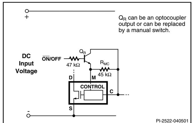
Figure 37. Active-off Remote ON/OFF. Maximum Duty Cycle Reduced.
