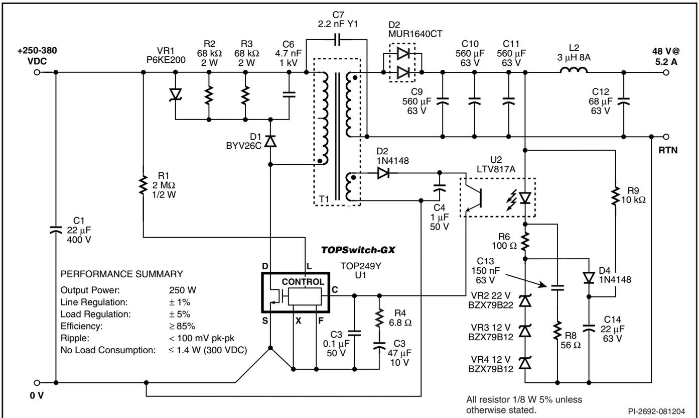
Figure 43. 250 W, 48 V Power Supply using TOP249.
