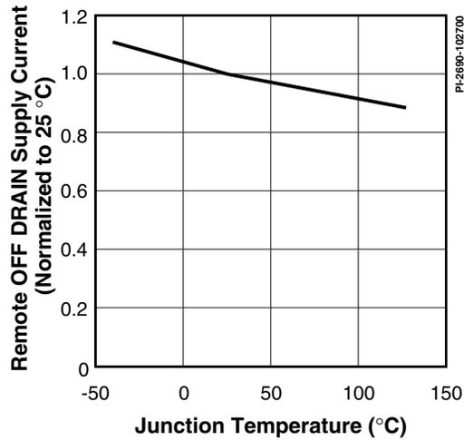
Figure 71. Remote OFF DRAIN Supply Current vs. Temperature.
