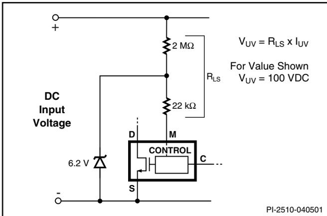
Figure 18. Line-Sensing for Under-Voltage Only (Overvoltage Disabled).
