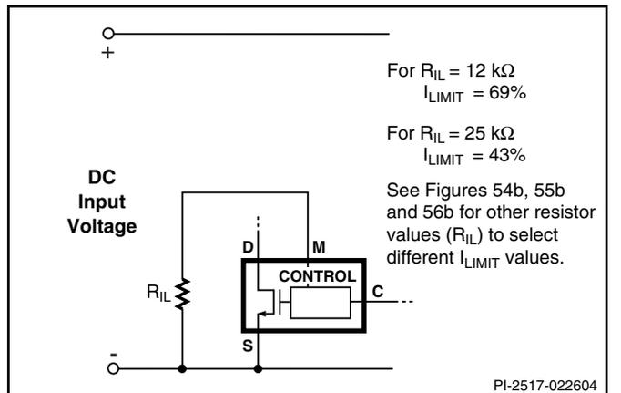
Figure 6. P/G Package Externally Set Current Limit.
