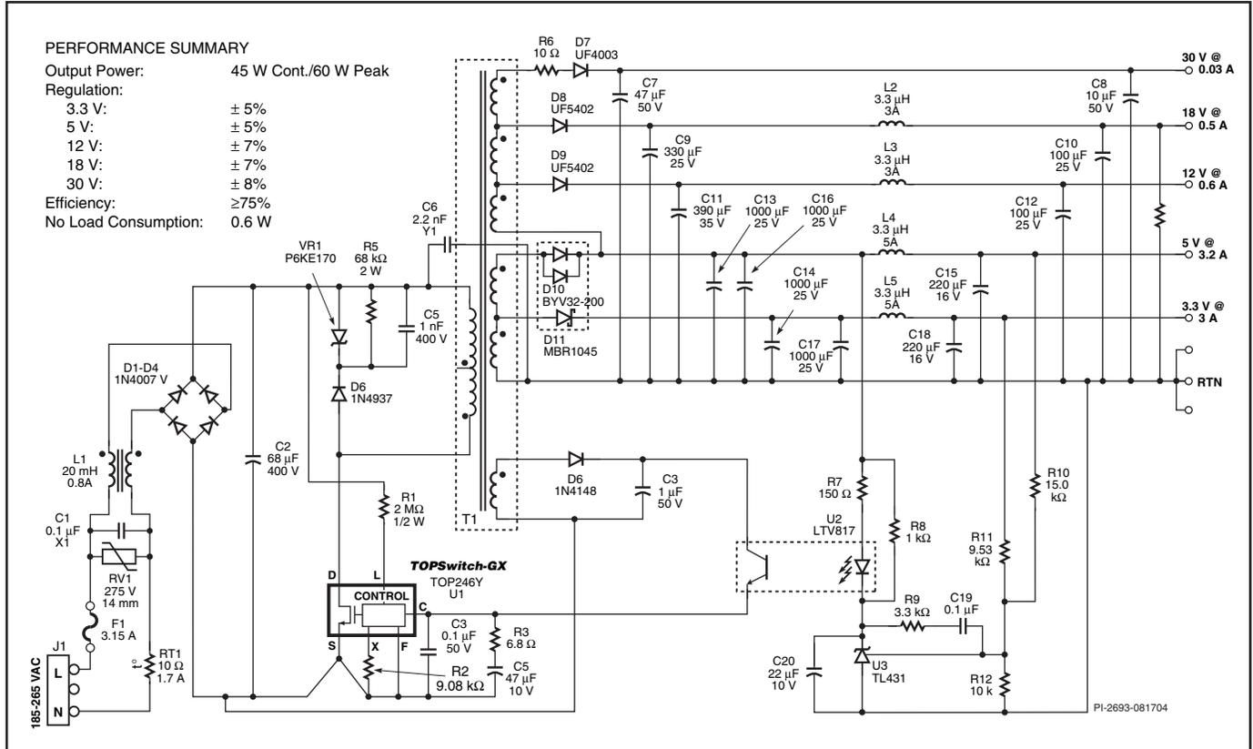
Figure 44. 60 W Multiple Output Power Supply using TOP246.
