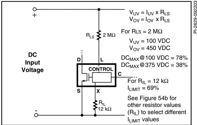
Figure 28. Line-Sensing and Externally Set Current Limit.
