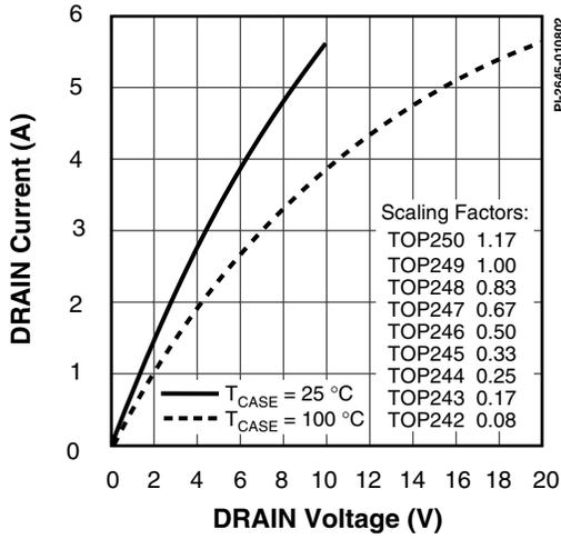
Figure 67. Output Characteristics.
