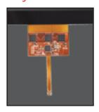
Fusion touch displays include an integrated touch controller system mounted directly on the flex tail (Chip on Flex). The Fusion controller runs Touch Revolution's proprietary firmware, capable of tracking at least two unambiguous touch points with a high report rate.
