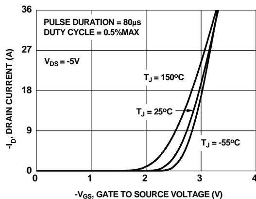
**Figure 5. Transfer Characteristics**
