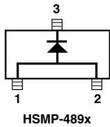
Figure 16. Internal Connections.
