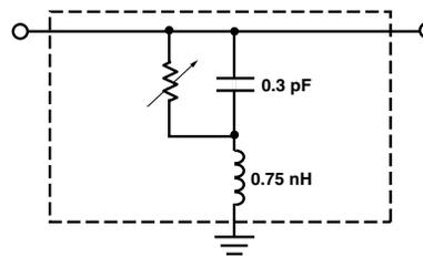
Figure 21. Equivalent Circuit.
