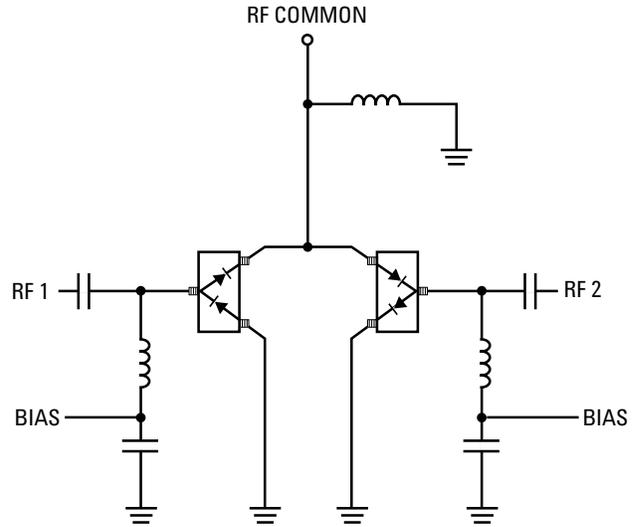
Figure 13. High Isolation SPDT Switch, Dual Bias.
