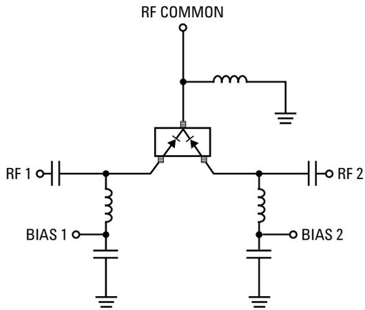
Figure 12. Simple SPDT Switch, Using Only Positive Current.
