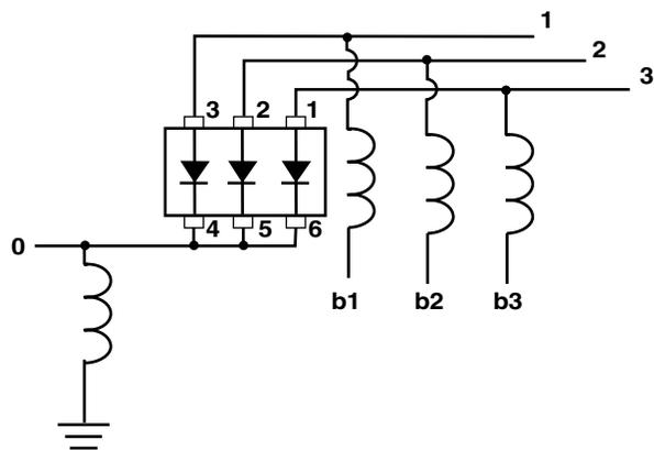
Figure 6. HSMF-389L used in a SP3T Switch.
