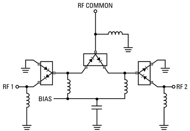
Figure 15. Very High Isolation SPDT Switch, Dual Bias.
