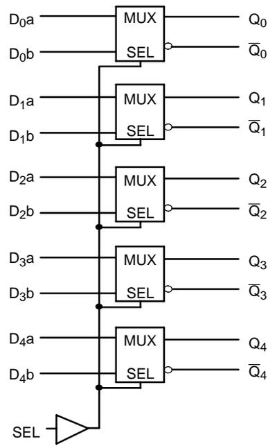
**Figure 2. Logic Diagram**
