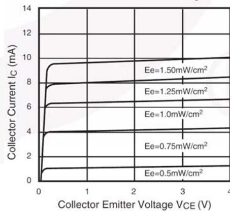
Figure 6. Collector Current vs. Collector Emitter Voltage
