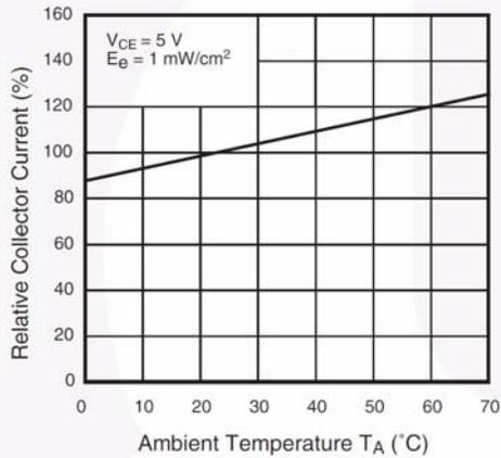
Figure 3. Relative Collector Current vs. Ambient Temperature
