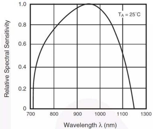
Figure 2. Spectral Sensitivity
