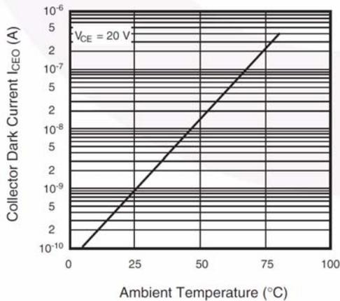
Figure 5. Collector Dark Current vs. Ambient Temperature
