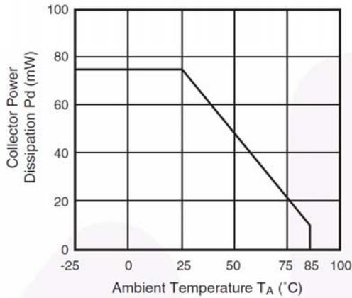
Figure 1. Collector Power Dissipation vs. Ambient Temperature
