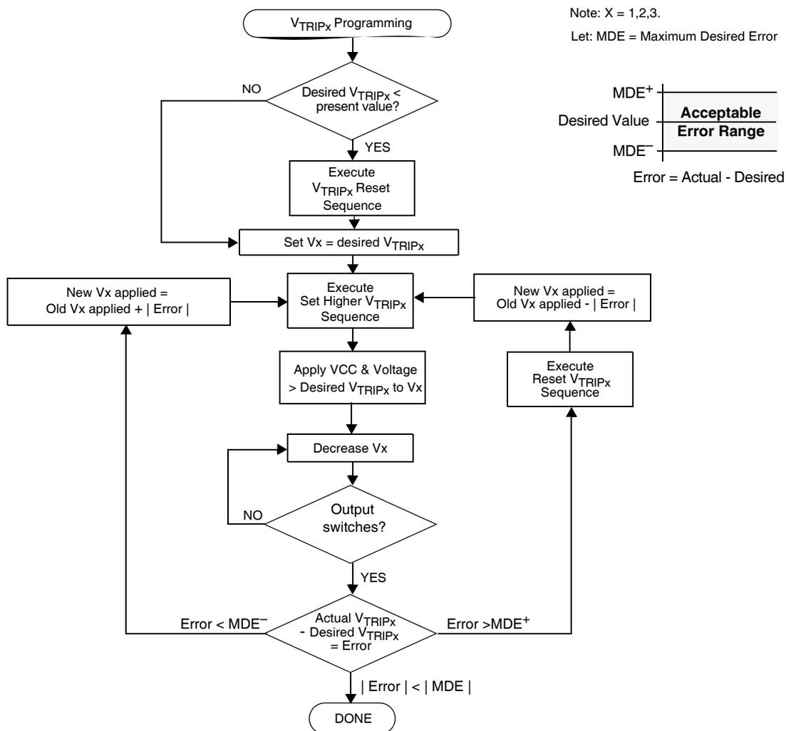
FIGURE 24.  $V_{TRIPx}$  SETTING/RESET SEQUENCE (X = 1,2,3)
