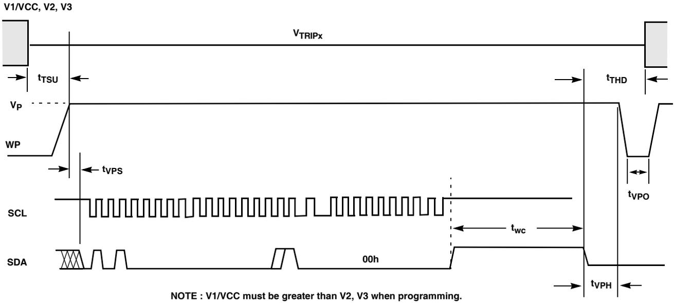
FIGURE 33. V<sub>TRIPX</sub> PROGRAMMING TIMING DIAGRAM (X = 1,2,3)
