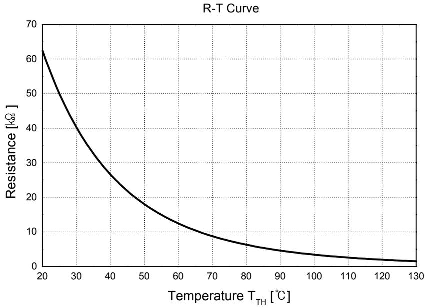
Fig. 6. R-T Curve of The Built-in Thermistor
