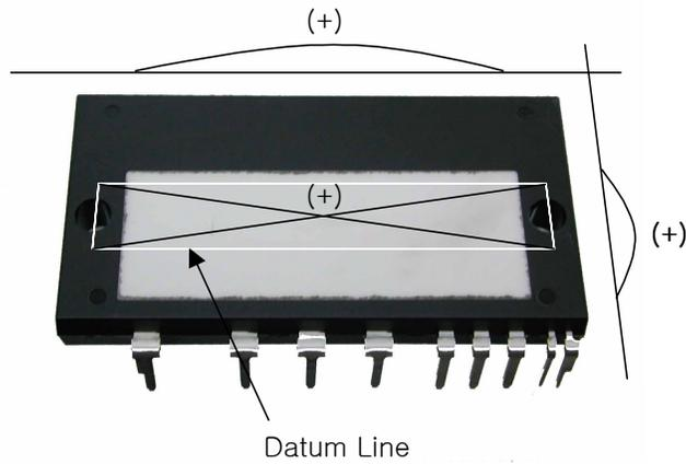
**Fig. 8. Flatness Measurement Position of The Ceramic Substrate**
