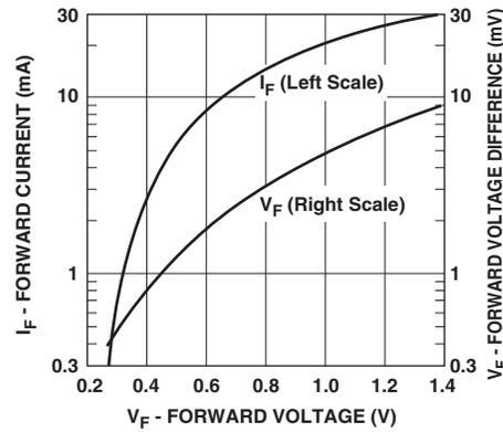
**Figure 5. Typical  $V_f$  Match, Pairs and Quads.**
