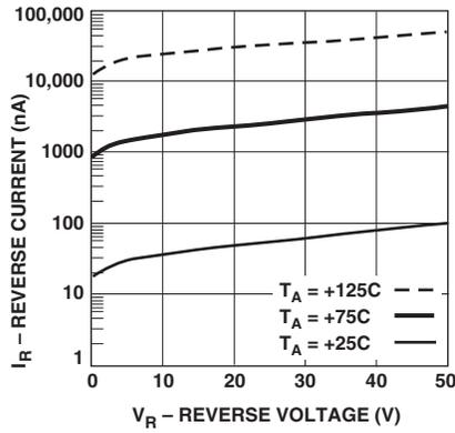
**Figure 2. Reverse Current vs. Reverse Voltage at Temperatures.**
