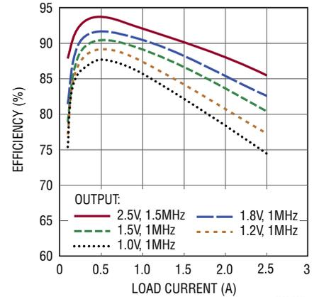
**Burst Mode Efficiency, 12V<sub>IN</sub>, 1.5V<sub>OUT</sub>**
