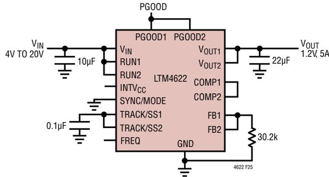
Figure 25. 4V<sub>IN</sub> to 20V<sub>IN</sub>, 1.2V Two Phase in Parallel 5A Design
