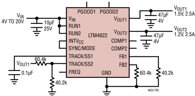
Figure 5. Example Schematic of Ratiometric Output Voltage Tracking
