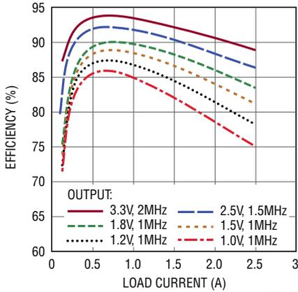
**Efficiency vs Load Current at 12V<sub>IN</sub>**
