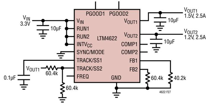
Figure 27. 3.3V<sub>IN</sub>, 1.5V and 1.2V Output at 2.5A Design with Output Coincident Tracking
