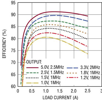
**Efficiency vs Load Current at 3.3V<sub>IN</sub>**
