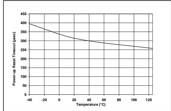
**FIGURE 2-3:** Power-up Reset Time Out vs. Temperature.
