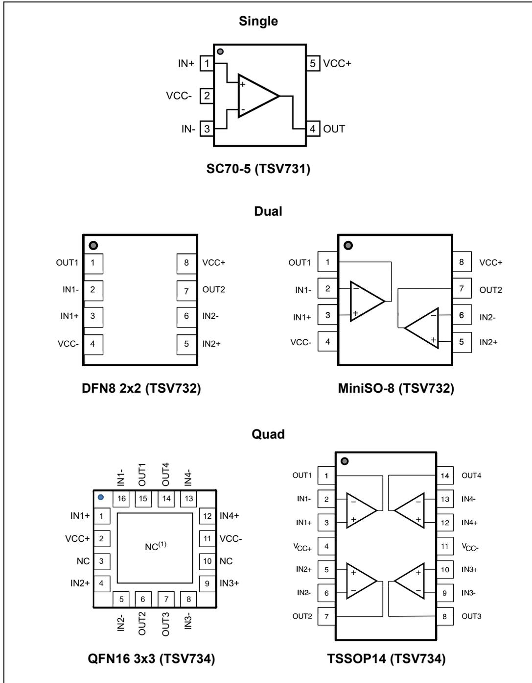
1. The exposed pads of the QFN16 3x3 can be connected to VCC- or left floating.
