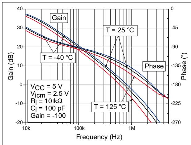
Figure 13. Closed-loop gain diagram vs. capacitive load
