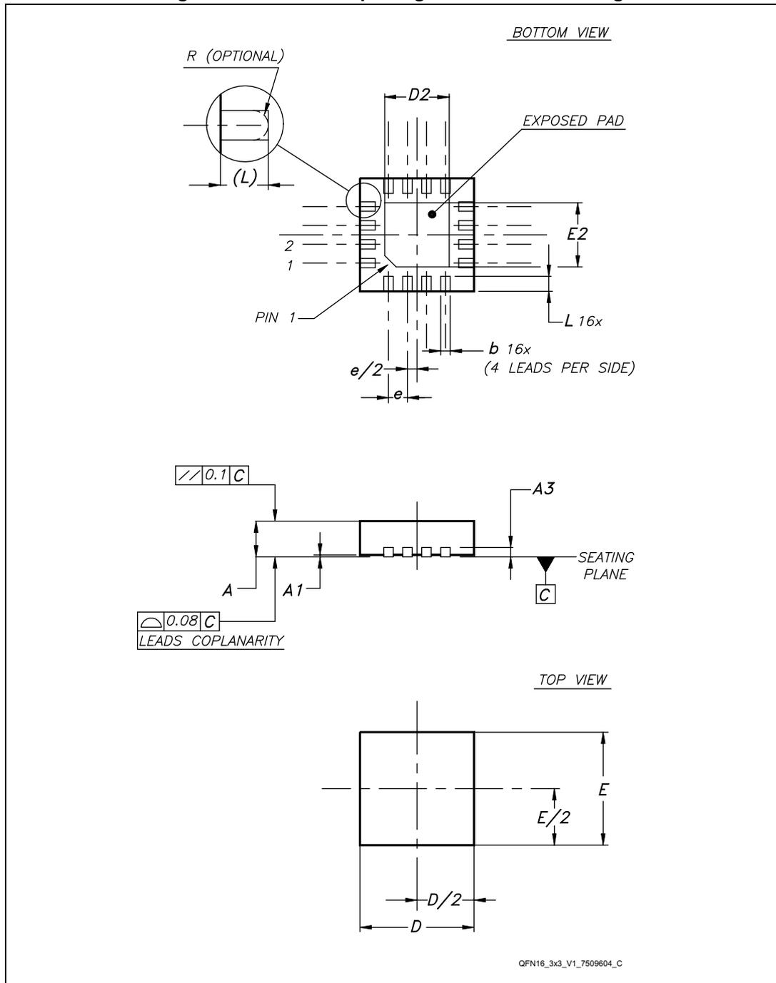
Table 10. QFN16 3x3 mm package mechanical data (pitch 0.5 mm)
