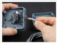
Remove the cable-clamp and clip the wires to remove the cable.
