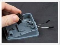
Feed the ends of the jumpers through the cable hole and re-install the switch.
