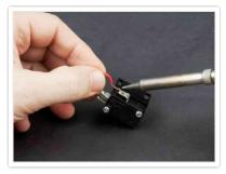
Remove the switch and use a soldering iron to de-solder the old wires.
