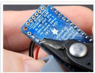
Solder one of the wires from the switch to one of the other Gnd holes, and clip the soldered wires close to the board.
