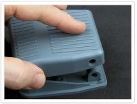
Position the spring between the two halves of the foot switch.
