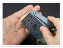
Locate and remove the small locking-pin near the front edge of the switch. It should fall out easily when you turn it over.
