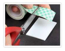
Cut a piece of double-sided foam tape about as wide as the plastic plate (1 3/4") and stick to one end of the plate.
