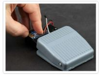
Cut another piece of tape to fit on the bottom side of the EZ-Key. Mount the EZ-Key to the top of the battery box. Keep to the left so you don't cover the ON/OFF switch.
