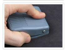
Press down on the top half of the switch to align the holes and insert the hinge pin. Make sure that the notch in the hinge pin is positioned to line up with the small locking pin you removed earlier.
