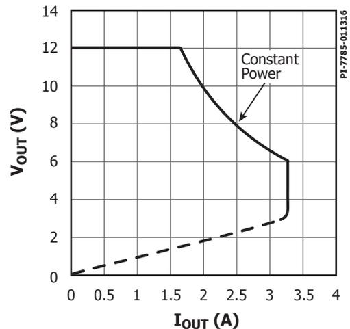
Figure 2. Output Characteristics.
