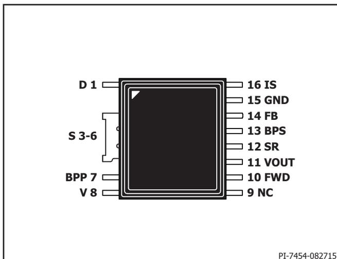
Figure 6. Pin Configuration.
