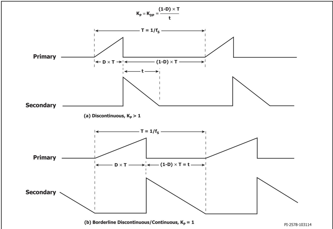
Figure 20. Discontinuous Mode Current Waveform,  $K_p \geq 1$ .
