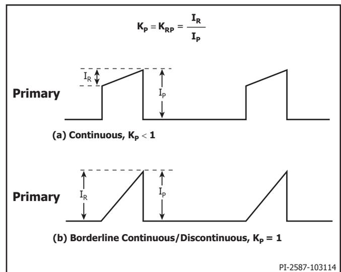
Figure 19. Continuous Mode Current Waveform,  $K_p \leq 1$ .
