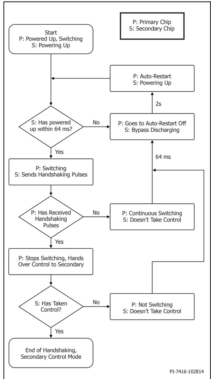
Figure 7. Primary-Secondary Handshake Flowchart.
