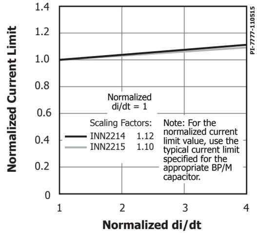
Figure 22. Standard Current Limit Vs.  $di/dt$ .
