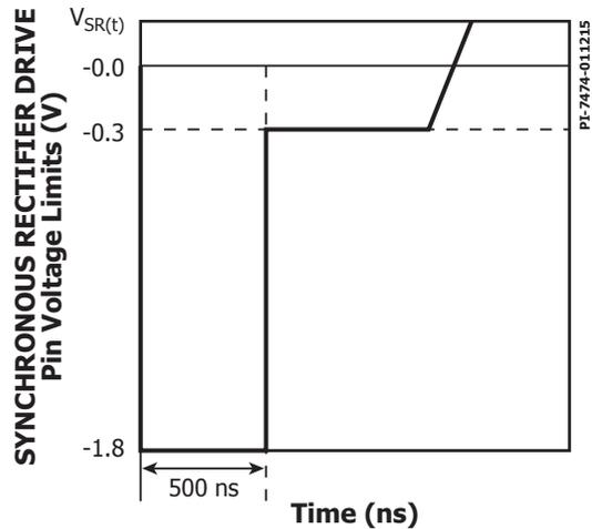
Figure 26. SYNCHRONOUS RECTIFIER DRIVE Pin Negative Voltage.
