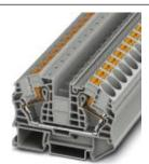
Feed-through terminal block, Connection method: Push-in connection, Cross section: 0.5 mm<sup>2</sup> - 25 mm<sup>2</sup>, AWG: 20 - 4, Width: 12.2 mm, Color: gray, Mounting type: NS 35/7,5, NS 35/15
