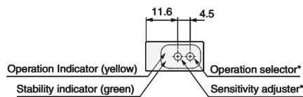
\*No sensitivity adjuster and operation selector with BGS reflective model
