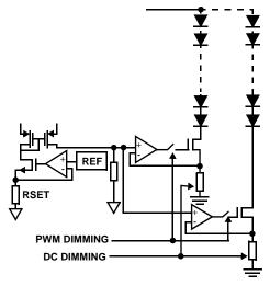
FIGURE 19. SIMPLIFIED CURRENT SOURCE CIRCUIT
