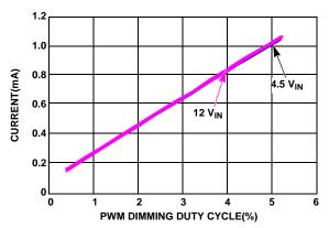
FIGURE 8. CURRENT LINEARITY vs LOW LEVEL PWM DIMMING DUTY CYCLE vs  $\mathbf{V}_{\mathrm{IN}}$
