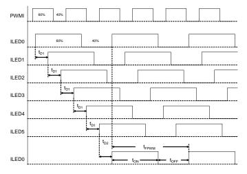
FIGURE 21. 6 EQUAL PHASE CHANNELS PHASE SHIFT ILLUSTRATION
