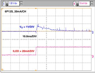
FIGURE 15. BOOST OUTPUT VOLTAGE WITH BRIGHTNESS CHANGE FROM 0% TO 100%,  $V_{\rm IN}$  = 12V, 6P12S AT 20mA/CHANNEL
