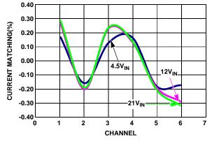
FIGURE 7. CHANNEL-TO-CHANNEL CURRENT MATCHING
