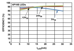
FIGURE 3. EFFICIENCY vs UP TO 30mA LED CURRENT (100% LED DUTY CYCLE) vs  $V_{\rm IN}$
