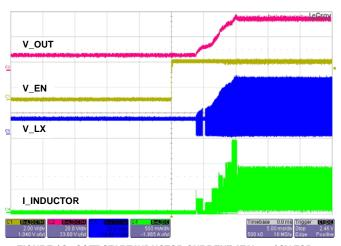
FIGURE 12. SOFT-START INDUCTOR CURRENT AT  $V_{\rm IN}$  = 12V FOR 6P12S AT 20mA/CHANNEL
