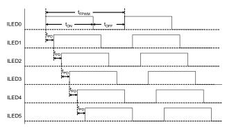
FIGURE 23. PHASE SHIFT WITH 7-BIT PROGRAMMABLE DELAY
