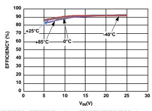
FIGURE 6. EFFICIENCY vs  $V_{\text{IN}}$  vs TEMPERATURE AT 20mA (100% LED DUTY CYCLE)
