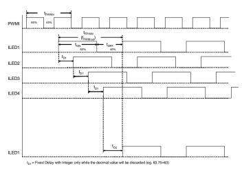
FIGURE 22. 4 EQUAL PHASE CHANNELS PHASE SHIFT ILLUSTRATION
