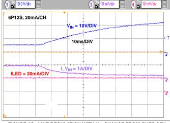
FIGURE 13. LINE REGULATION WITH  $V_{\rm IN}$  CHANGE FROM 6V TO 26V, 6P12S AT 20mA/CHANNEL
