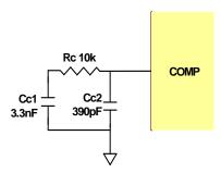
FIGURE 40. COMPENSATION CIRCUIT
