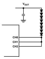
FIGURE 37. GANGING MULTIPLE CHANNELS FOR HIGH CURRENT APPLICATIONS
