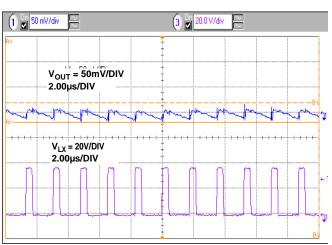
FIGURE 10. V<sub>OUT</sub> RIPPLE VOLTAGE, V<sub>IN</sub> = 12V, 6P12S AT 20mA/CHANNEL
