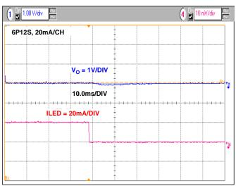
FIGURE 16. BOOST OUTPUT VOLTAGE WITH BRIGHTNESS CHANGE FROM 100% TO 0%, V<sub>IN</sub> = 12V, 6P12S AT 20mA/CHANNEL
