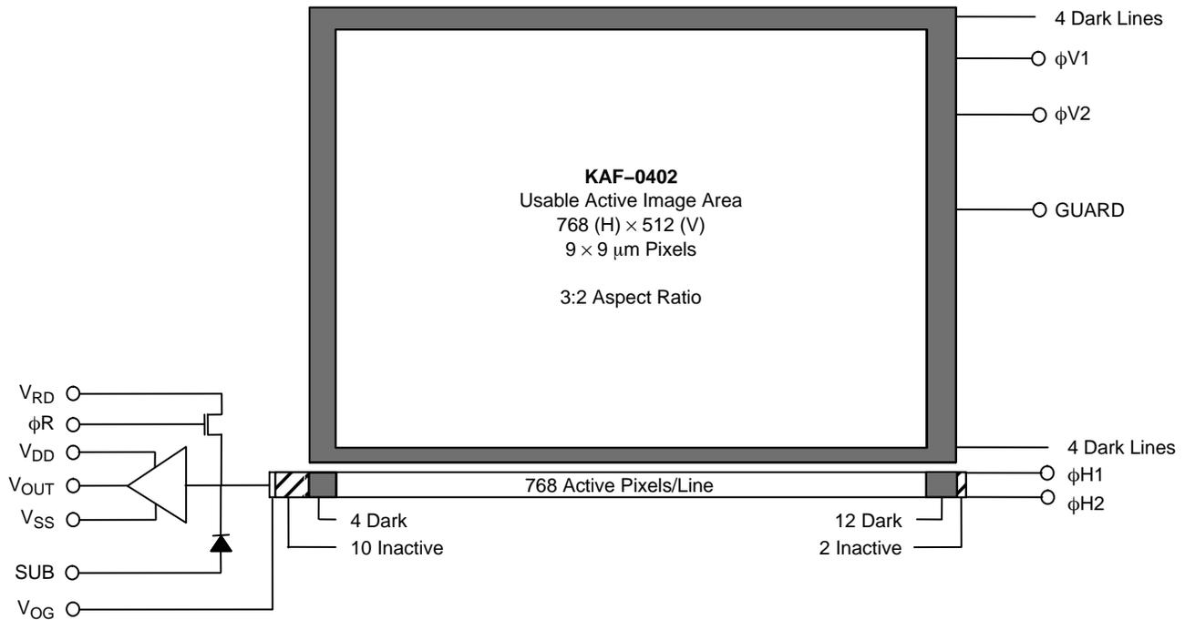
**Figure 2. Block Diagram**
