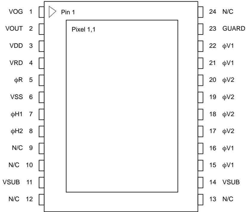
Figure 5. Pinout Diagram
