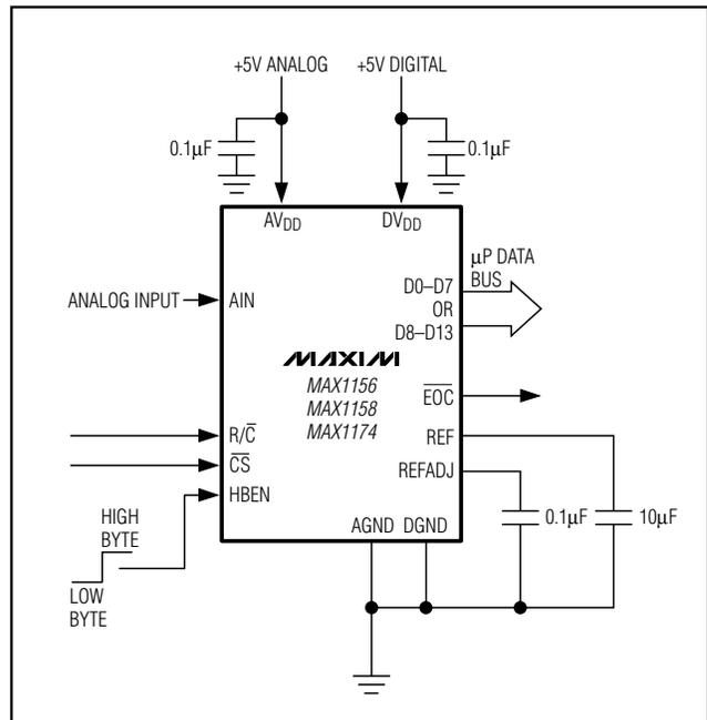
Figure 3. Typical Application Circuit for the MAX1156/MAX1158/MAX1174
