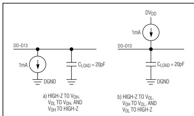
Figure 1. Load Circuits
