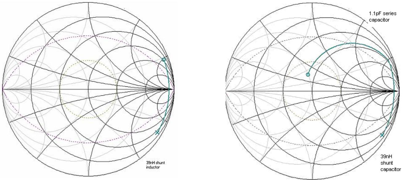
**Figure 9. Plotting the Shunt Inductor and Series Capacitor**
