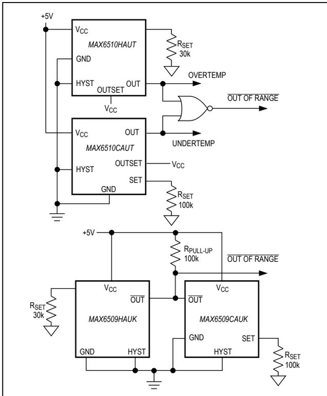
Figure 5. Temperature-Window Detector
