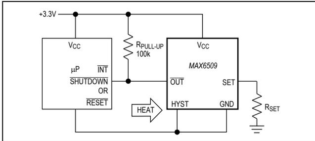
Figure 2. Microprocessor Alarm/Reset
