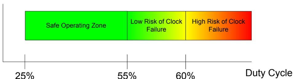
**Figure 19.2. Interpreting Oscillation Robustness (Duty Cycle) Test Results**
