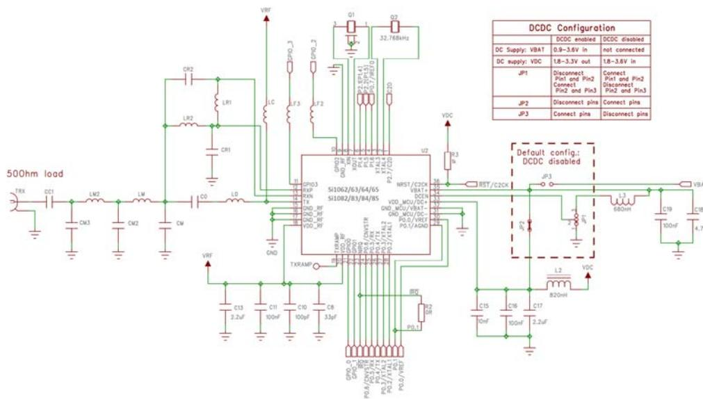
Figure 1.2. Si106x/108x RX/TX Direct-Tie Application Example
