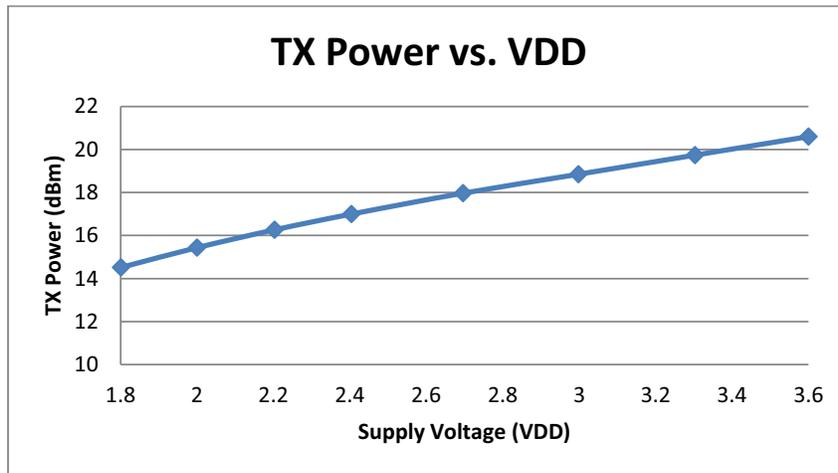
Figure 24.3. +20 dBm TX Power vs. VDD
