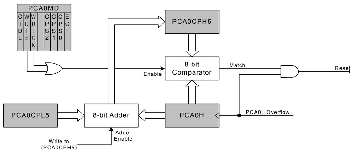
**Figure 32.11. PCA Module 5 with Watchdog Timer Enabled**
