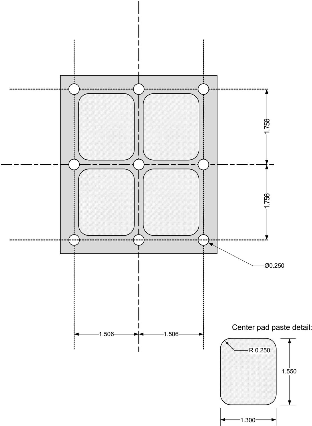
Figure 3.6. QFN-36 PCB Stencil and Via Placement
