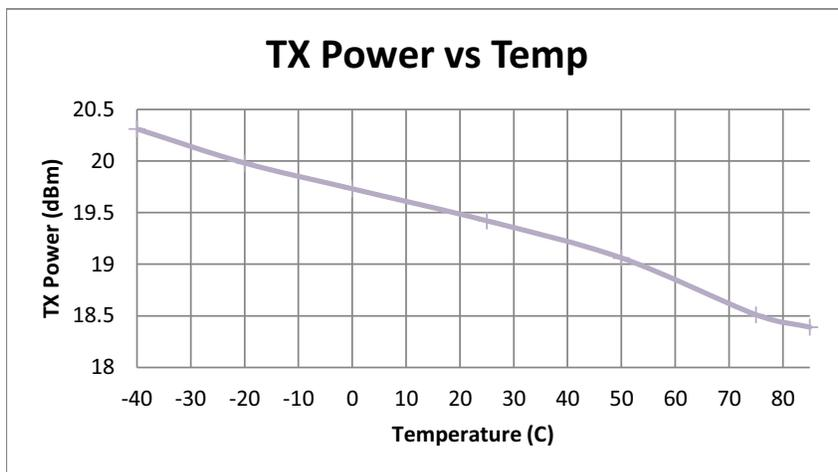
Figure 24.4. +20 dBm TX Power vs. Temp
