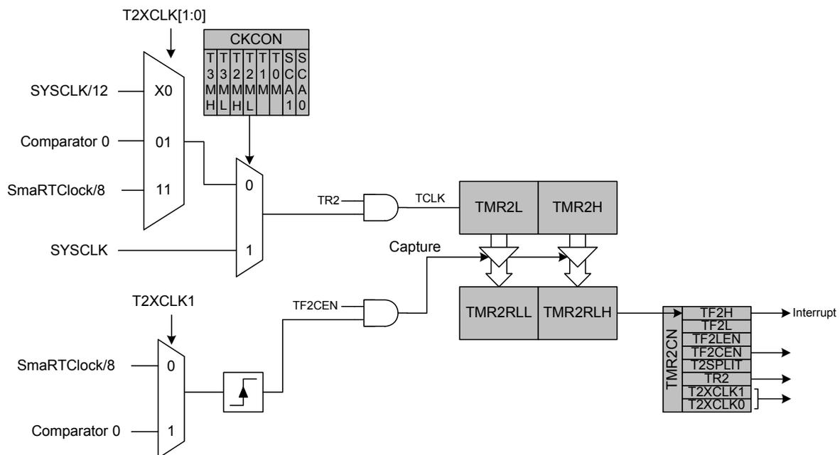
Figure 31.6. Timer 2 Capture Mode Block Diagram
