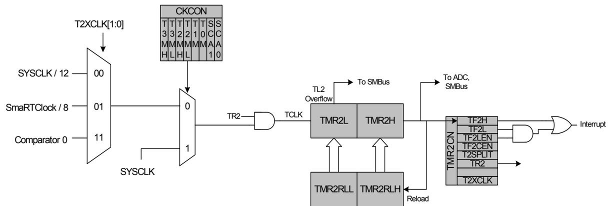
Figure 31.4. Timer 2 16-Bit Mode Block Diagram
