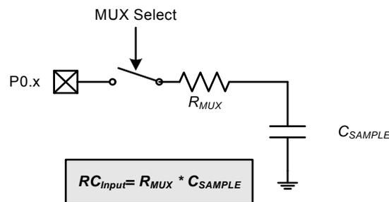
**Note:** The value of  $C_{SAMPLE}$  depends on the PGA Gain. See Table 4.9 for details.
