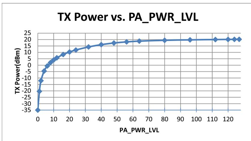
Figure 24.2. +20 dBm TX Power vs. PA\_PWR\_LVL
