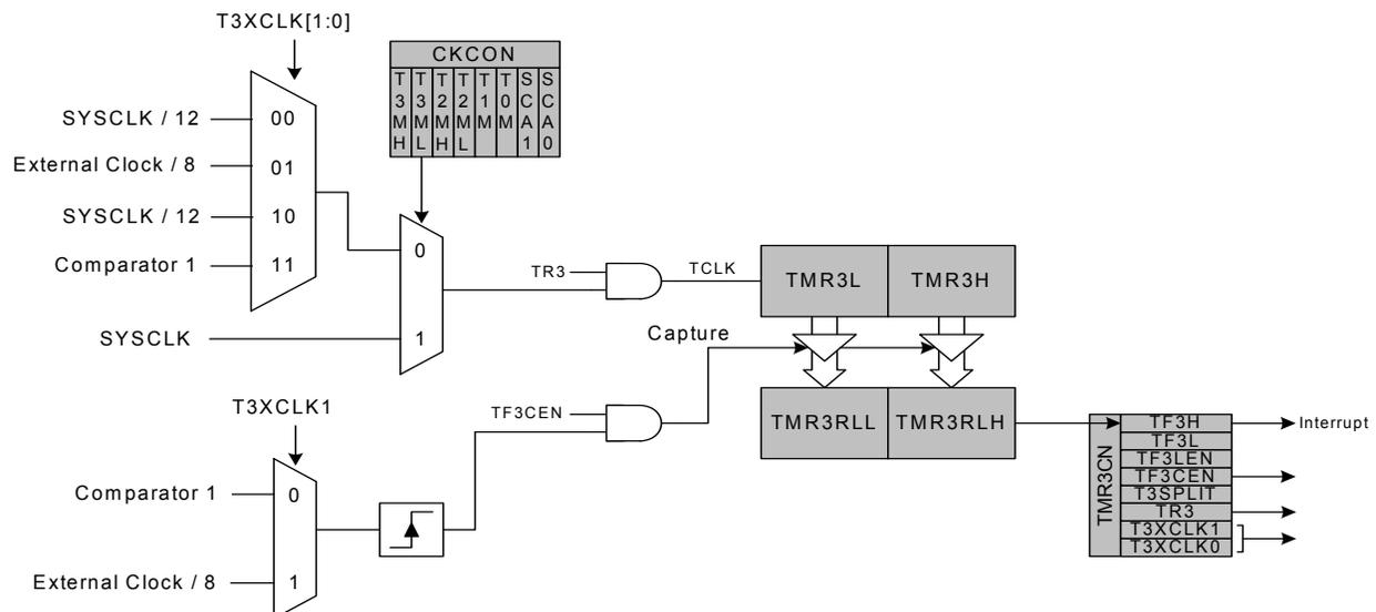
Figure 31.9. Timer 3 Capture Mode Block Diagram
