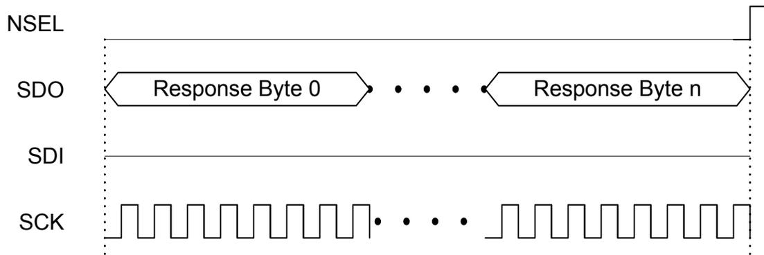
**Figure 21.3. SPI Read Command—Clock Out Read Data**
