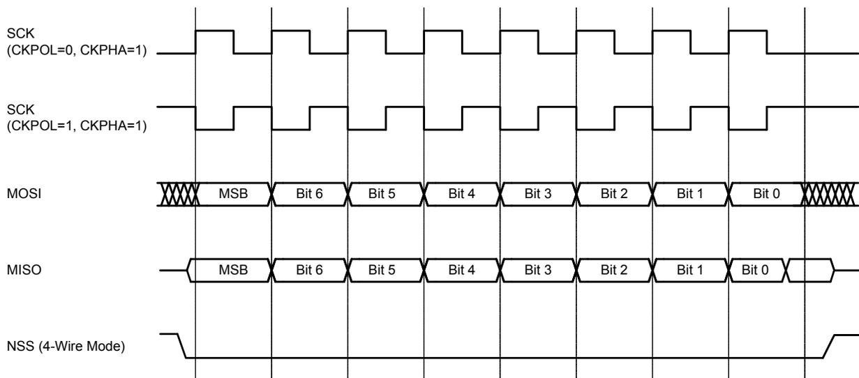
**Figure 30.7. Slave Mode Data/Clock Timing (CKPHA = 1)**
