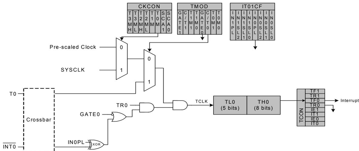
**Figure 31.1. T0 Mode 0 Block Diagram**
