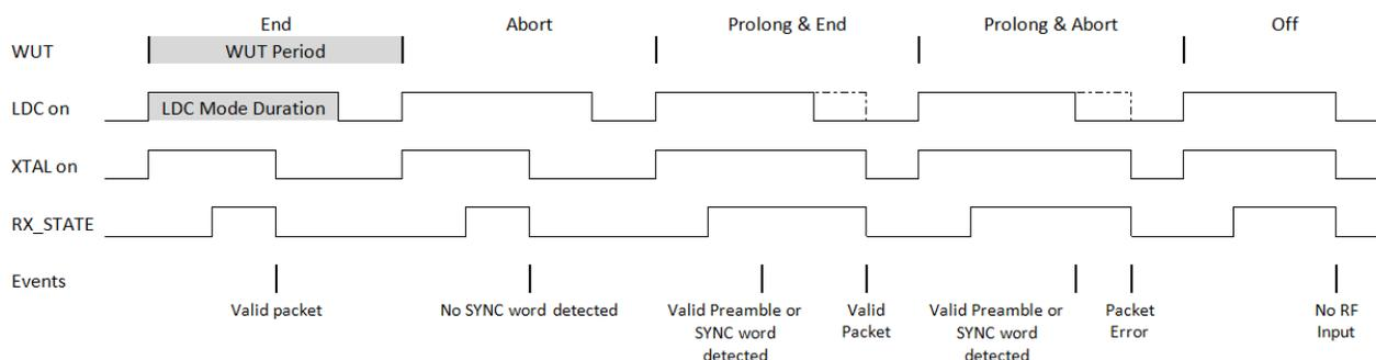
**Figure 27.2. Low Duty Cycle Mode for RX**
