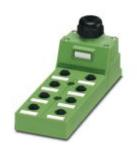
Sensor/actuator box, Connection method: M12 socket Plastic, Number of slots: 6, Number of positions: 4, Slot assignment: Single, Status indication: Yes, pnp; Master cable connection: Pluggable screw connection 90°, Shielding: No
