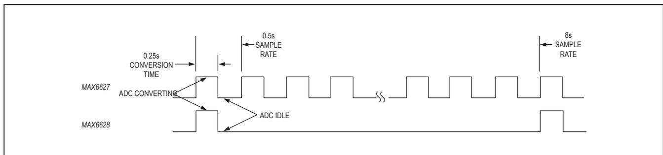
Figure 1. Free-Running Conversion Time and Rate Relationships
