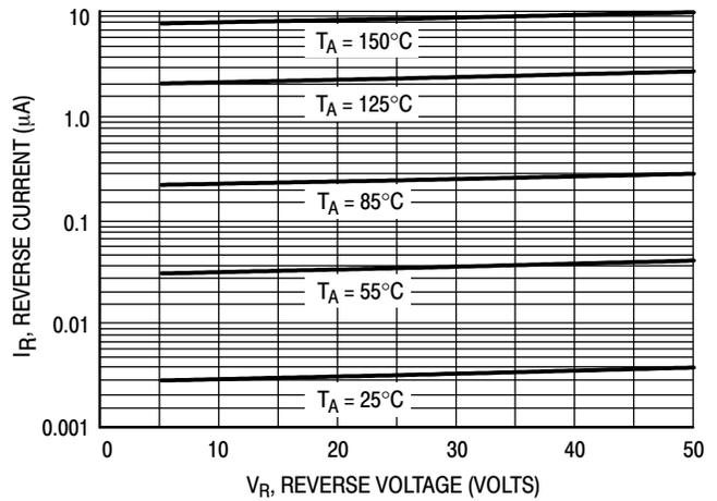
**Figure 3. Leakage Current**
