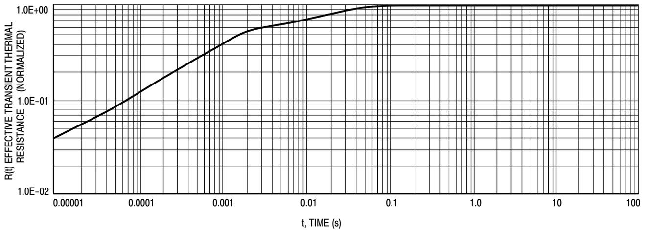
Figure 9. Transient Thermal Response ( $R_{\theta JC}$ )
