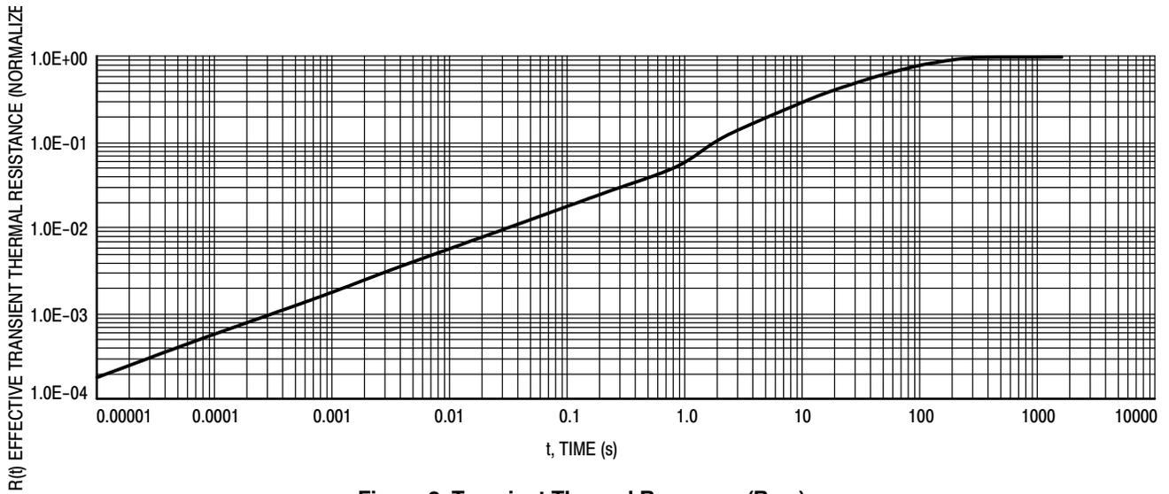
Figure 8. Transient Thermal Response ( $R_{\theta JA}$ )
