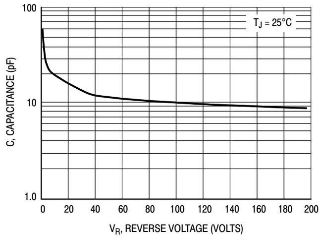
Figure 7. Typical Capacitance (Per Leg)
