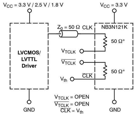
\*RTIN, Internal Input Termination Resistor
