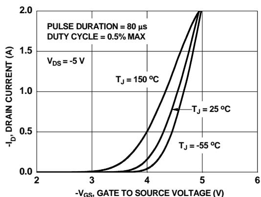
Figure 5. Transfer Characteristics
