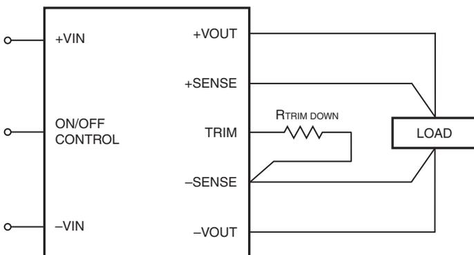
Figure 9. Trim Connections To Decrease Output Voltages
