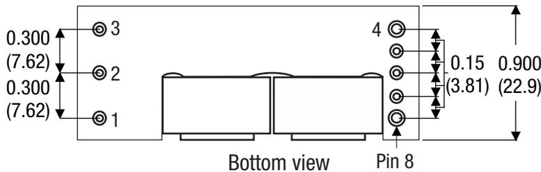
Standard pin length is shown. Please refer to the Part Number Structure for special order pin lengths.
