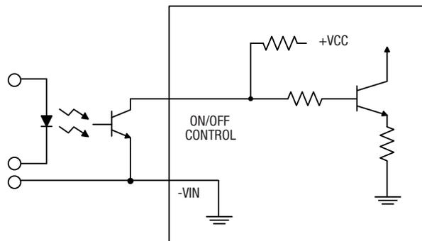
Figure 8. Driving the On/Off Control Pin (suggested circuit)
