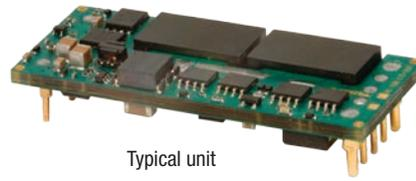
For efficient, fully isolated DC power in the smallest space, the UCE open frame DC-DC converter series fit in industry-standard “eighth brick” outline dimensions and mounting pins (on quarter-brick pinout).
