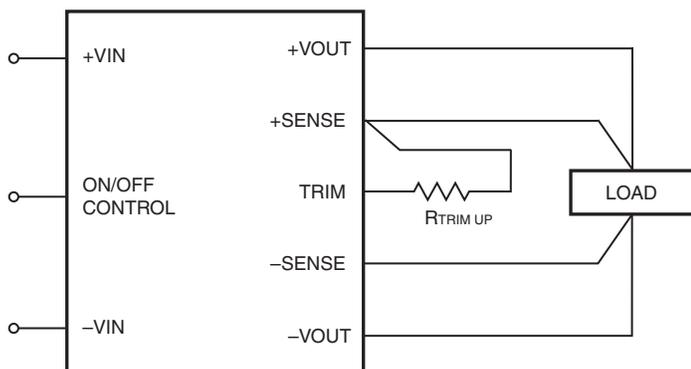
Figure 7. Trim Connections To Increase Output Voltages
