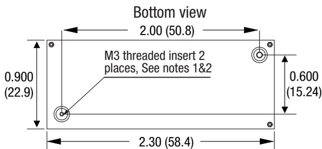
1. M3 screw used to bolt unit's baseplate to other surfaces (such as heatsink) must not exceed 0.118" (3mm) depth below the surface of baseplate
