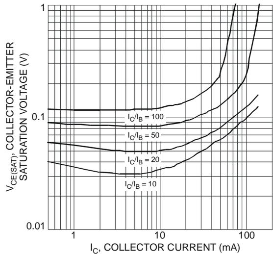
Fig. 7 Typical Collector-Emitter Saturation Voltage vs. Collector Current
