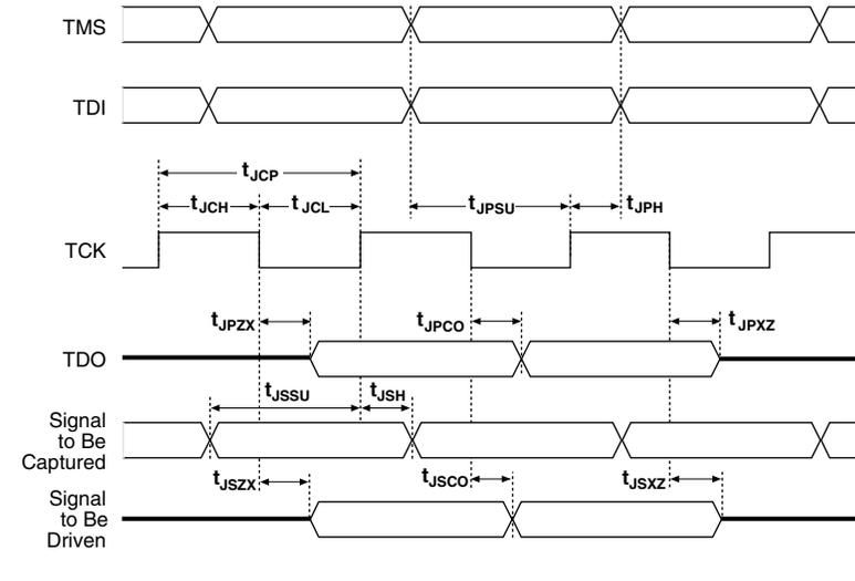
[Table 10](#) shows the JTAG timing parameters and values for FLEX 6000 devices.
