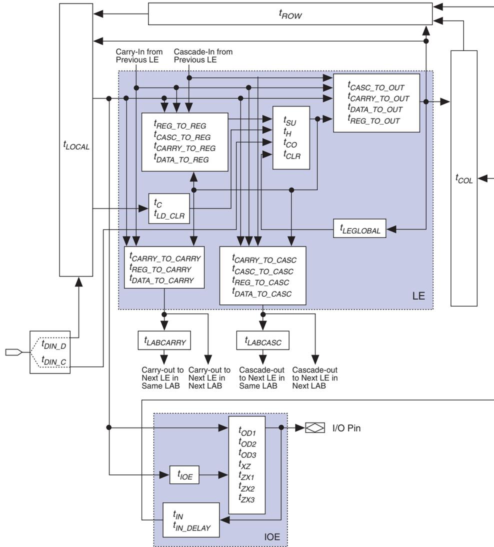
Tables 19 through 21 describe the FLEX 6000 internal timing microparameters, which are expressed as worst-case values. Using hand calculations, these parameters can be used to estimate design performance. However, before committing designs to silicon, actual worst-case performance should be modeled using timing simulation and timing analysis. Tables 22 and 23 describe FLEX 6000 external timing parameters.
