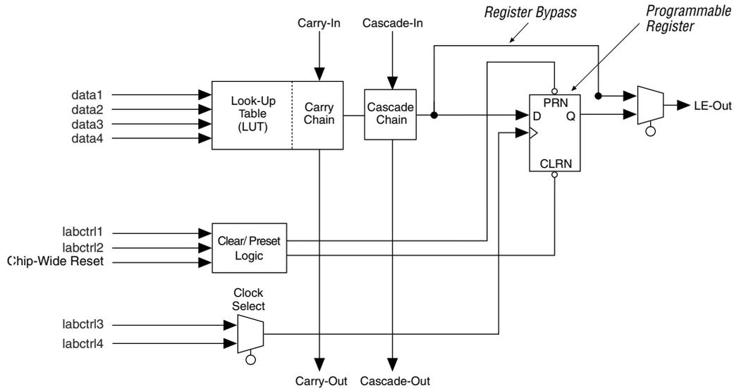
The programmable flipflop in the LE can be configured for D, T, JK, or SR operation. The clock and clear control signals on the flipflop can be driven by global signals, general-purpose I/O pins, or any internal logic. For combinatorial functions, the flipflop is bypassed and the output of the LUT drives the outputs of the LE. The LE output can drive both the local interconnect and the FastTrack Interconnect.
