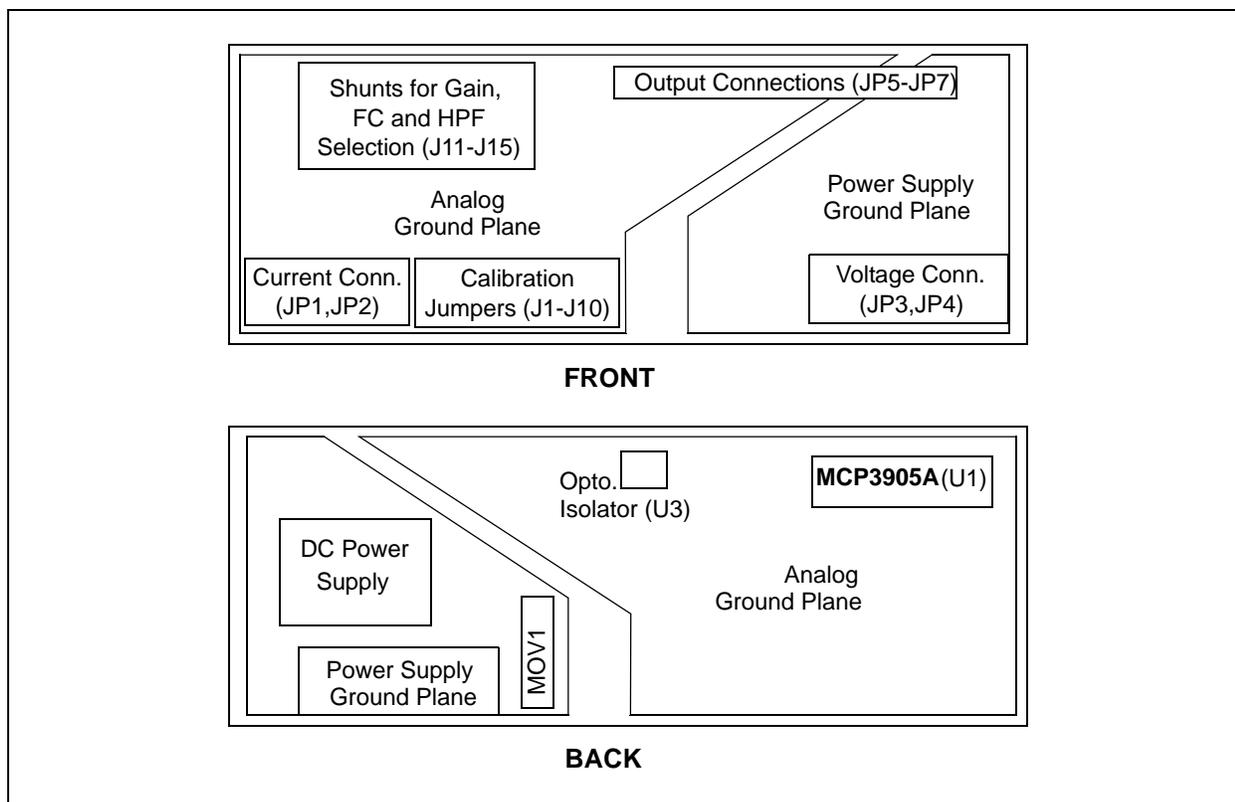
**FIGURE 2-3:** MCP3905A/06A Energy Meter Reference Design Block Diagram.
