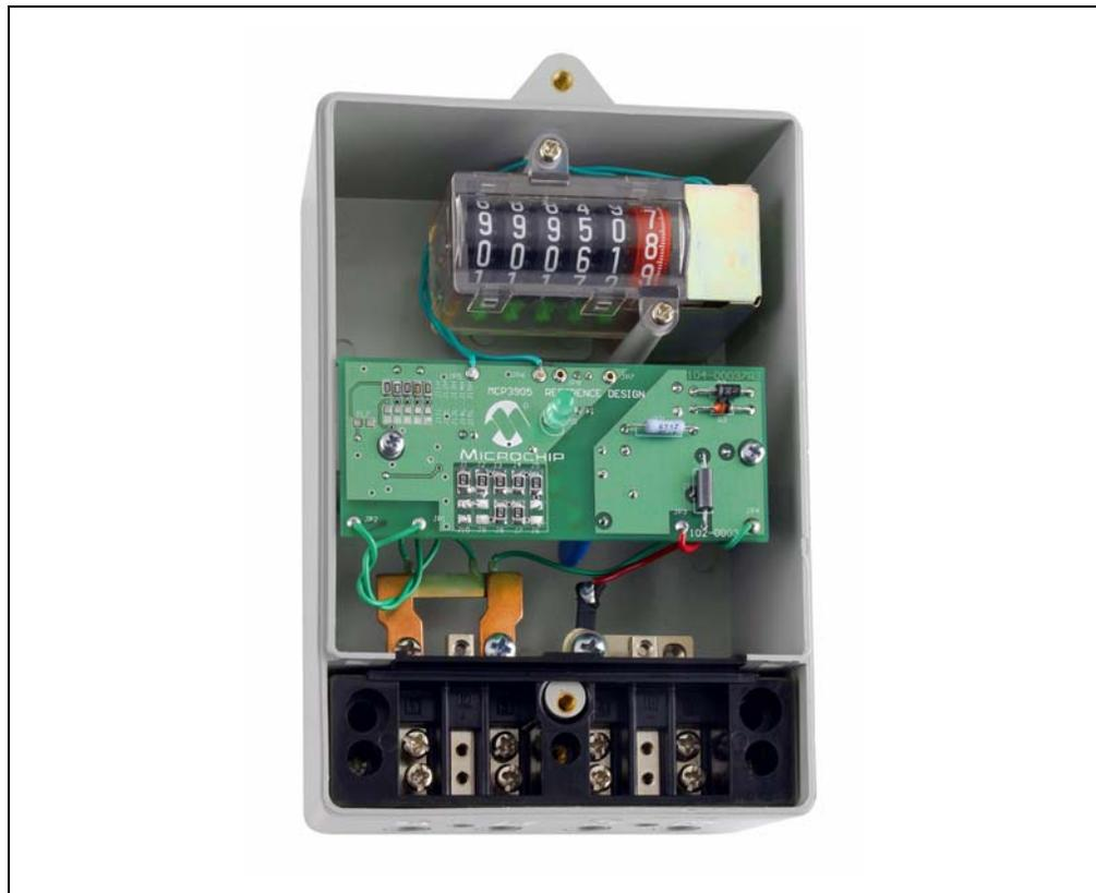
**FIGURE 2-2:** Photograph of Complete, Stand-Alone MCP3905A Energy Meter.
