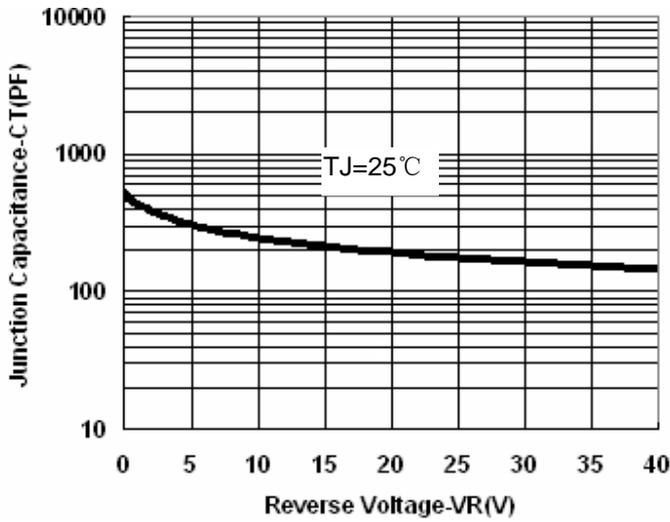
Fig.1-Typical Junction Capacitance
