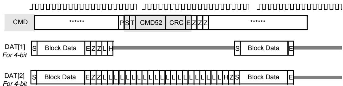
Figure 32. SDIO ReadWait Timing Diagram
