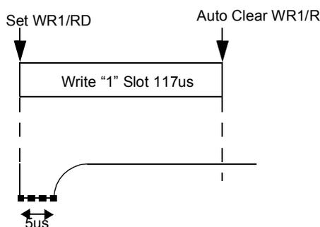
Figure 48. Write 1 Timing
