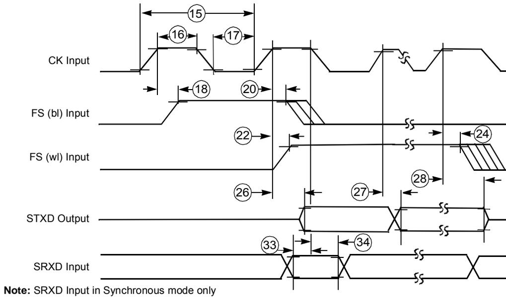
Figure 44. SSI Transmitter External Clock Timing Diagram
