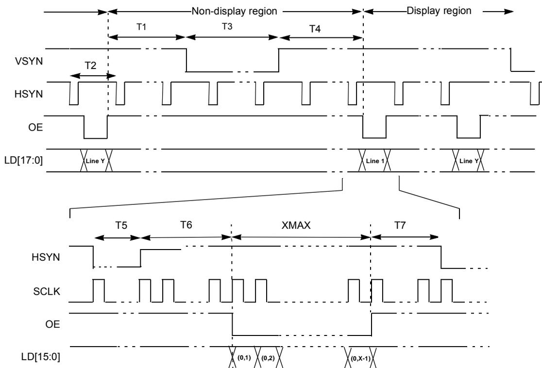
Figure 20. 4/8/12/16/18 Bit/Pixel TFT Color Mode Panel Timing
