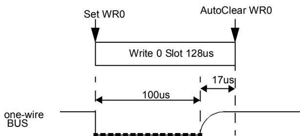
Figure 47. Write 0 Timing
