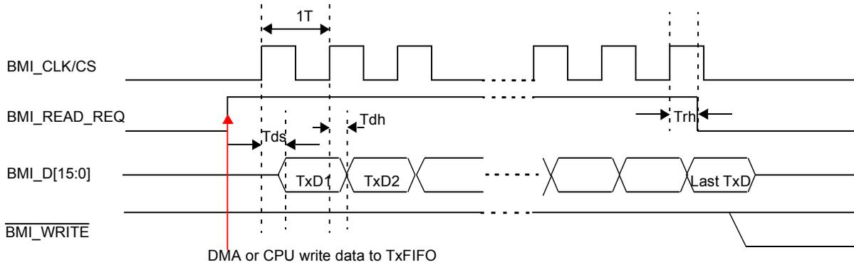
**Figure 8. BMI Drives Clock, MMD Read BMI Timing
