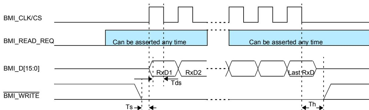
**Figure 7. MMD (ATI) Drives Clock, MMD Write BMI Timing**
