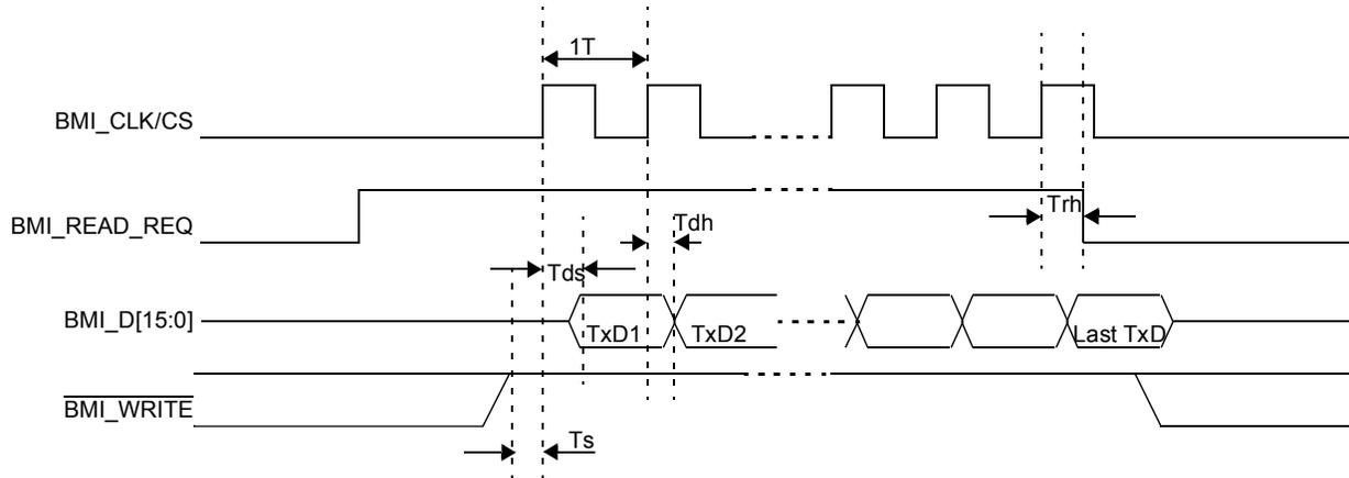
**Figure 6. MMD (ATI) Drives Clock, MMD Read BMI Timing
