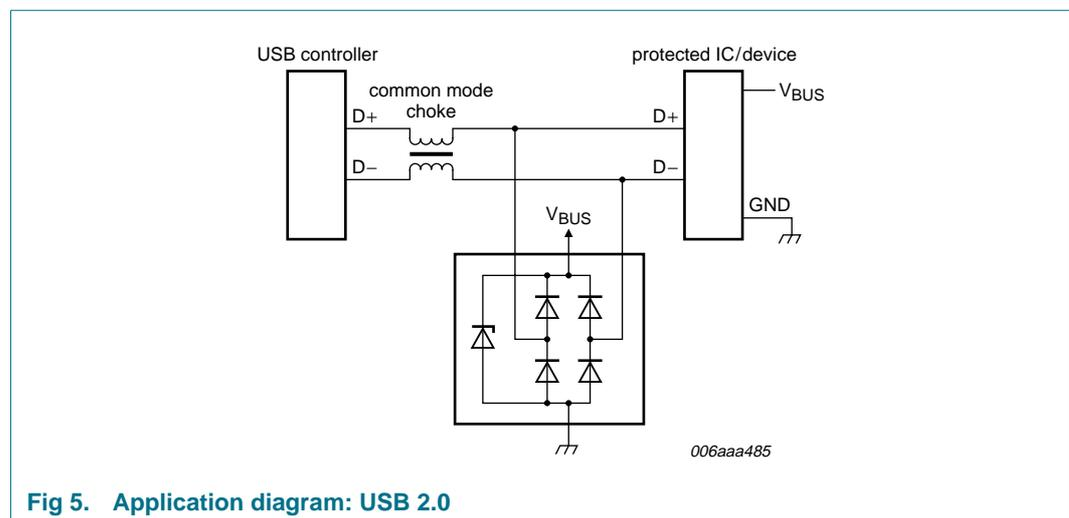
Fig 5. Application diagram: USB 2.0
