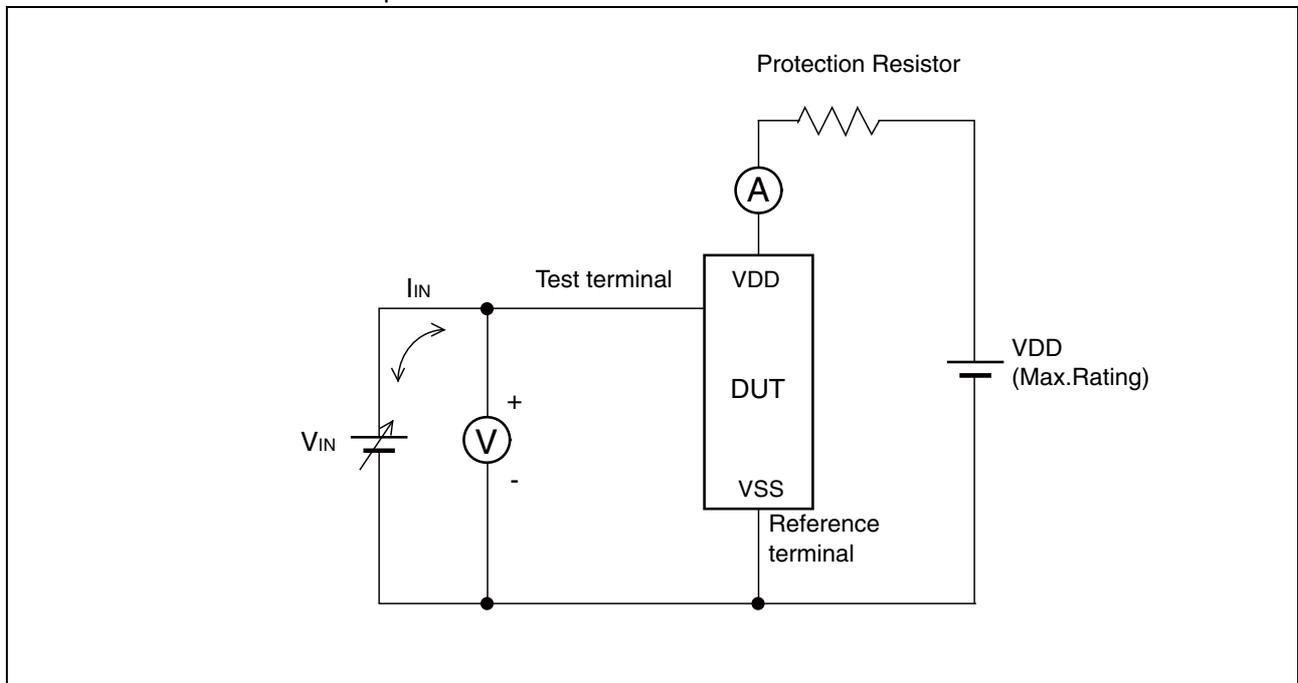
Note : The voltage  $V_{IN}$  is increased gradually and the current  $I_{IN}$  of 300 mA at maximum shall flow.
