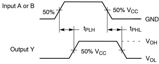
**Figure 3. Switching Waveforms**
