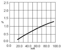
Relative Luminous Flux vs Forward Current
