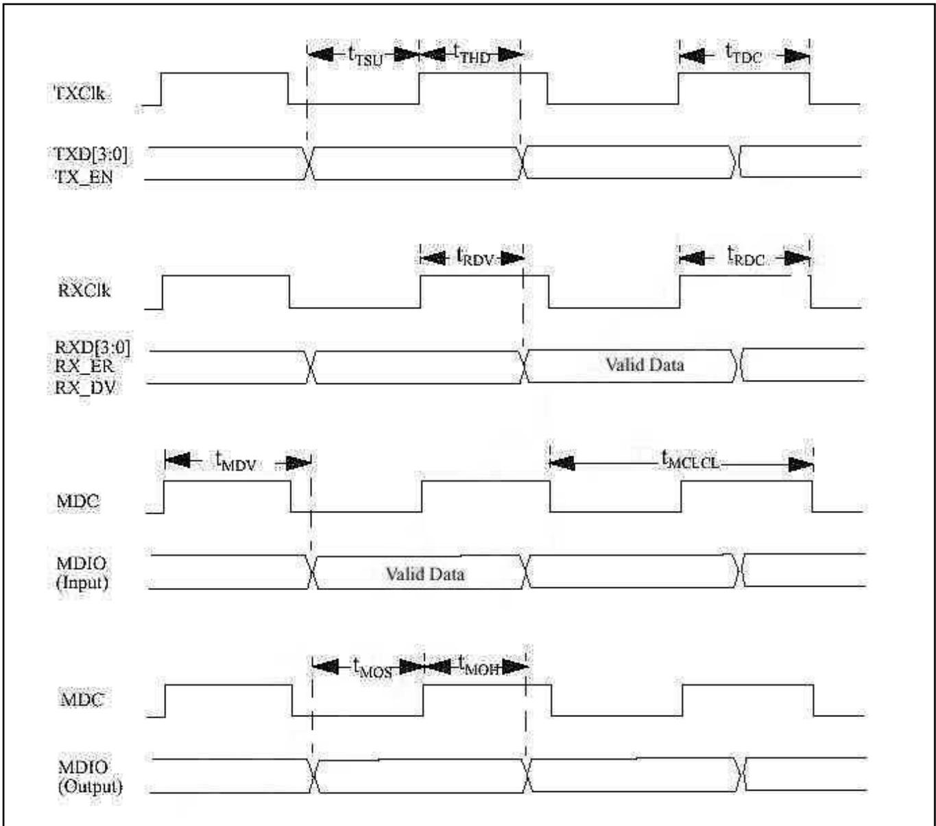
**SERIAL PORT MODE 0 TIMING CHARACTERISTICS (Note 1)**(V<sub>CC3</sub> = 3.0V to 3.6V, V<sub>CC1</sub> = 1.8V ±10%, T<sub>A</sub> = -40°C to +85°C.)
