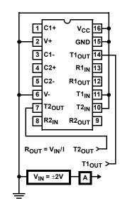
FIGURE 8. POWER-OFF SOURCE RESISTANCE CONFIGURATION
