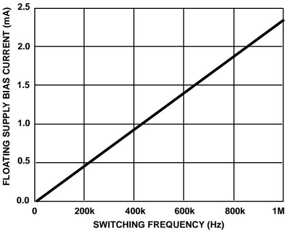
FIGURE 8. I<sub>AHB</sub>, I<sub>BHB</sub> NO-LOAD FLOATING SUPPLY BIAS CURRENT vs FREQUENCY
