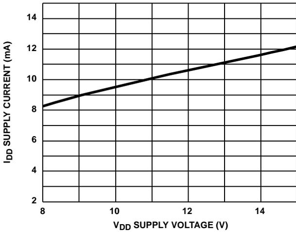
FIGURE 4. QUIESCENT I<sub>DD</sub> SUPPLY CURRENT vs V<sub>DD</sub> SUPPLY VOLTAGE
