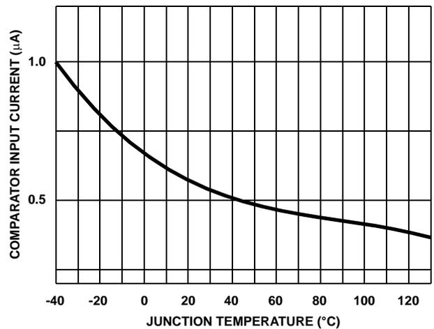
FIGURE 9. COMPARATOR INPUT CURRENT I<sub>L</sub> vs TEMPERATURE AT V<sub>CM</sub> = 5V
