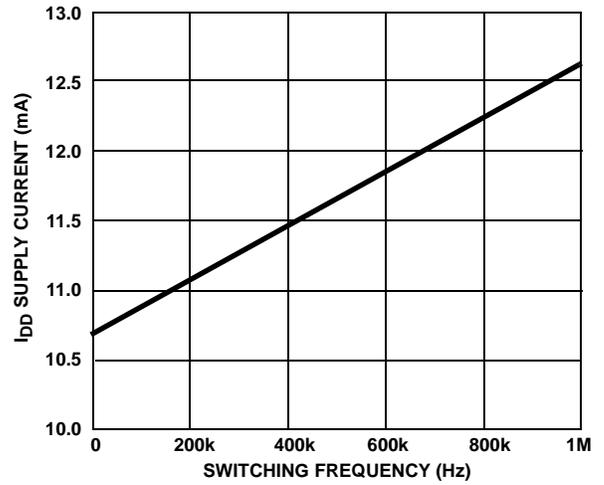
FIGURE 5. I<sub>DD0</sub> NO-LOAD I<sub>DD</sub> SUPPLY CURRENT vs FREQUENCY (Hz)
