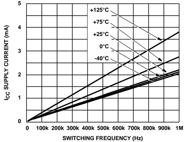
FIGURE 7. I<sub>CC0</sub>, NO-LOAD I<sub>CC</sub> SUPPLY CURRENT vs FREQUENCY (Hz) TEMPERATURE
