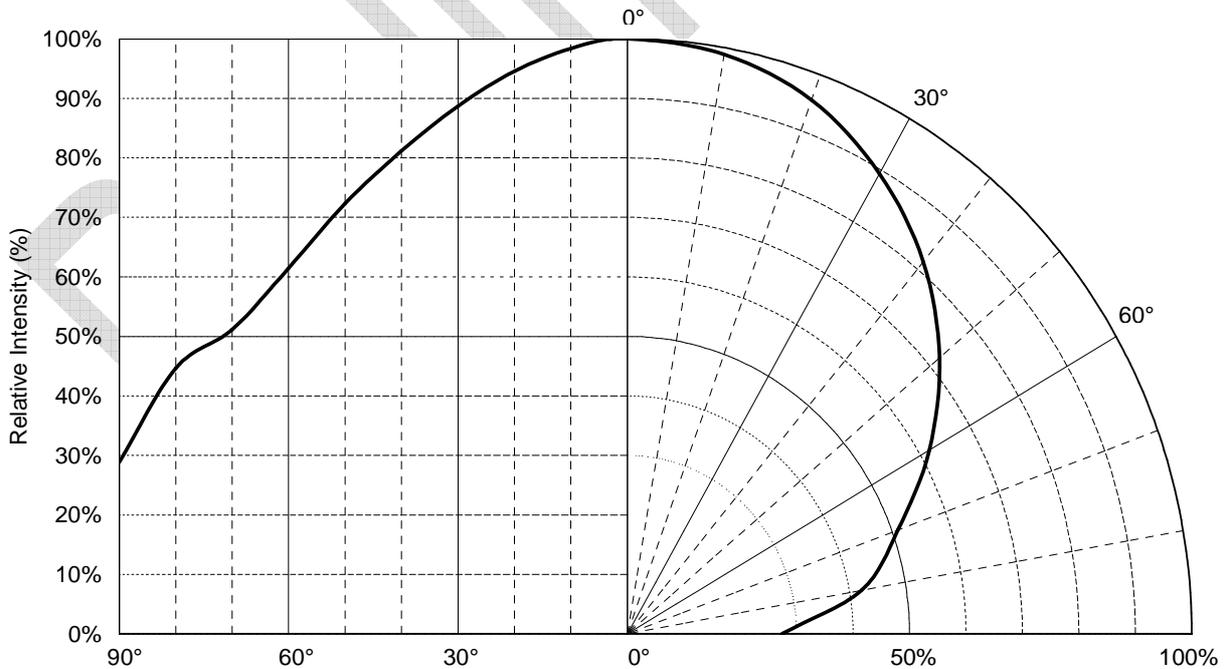
Fig 2. Radiation Characteristics
