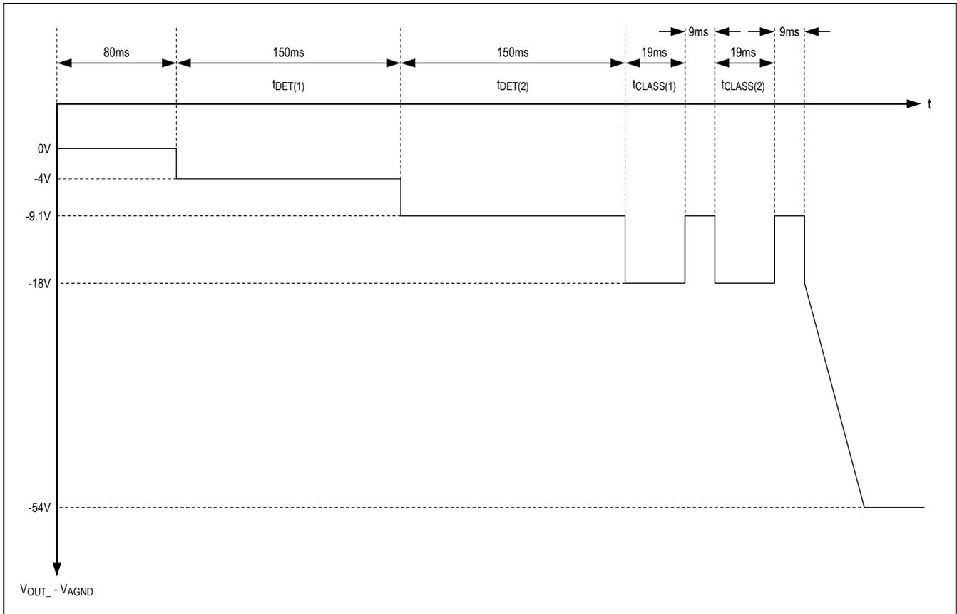
Figure 2. Detection, 2-Event Classification, and Port Power-Up Sequence
