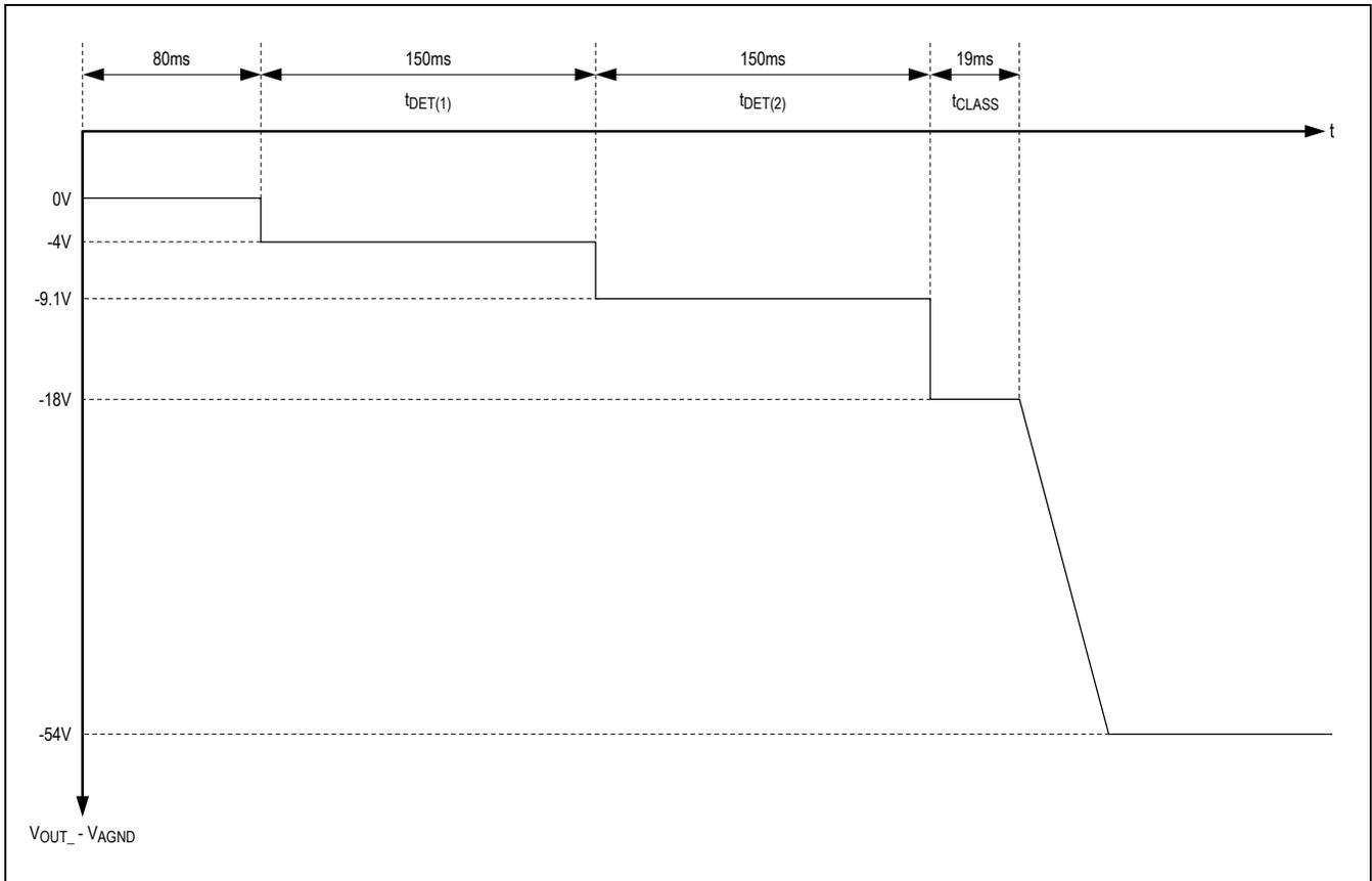
Figure 1. Detection, Classification, and Port Power-Up Sequence
