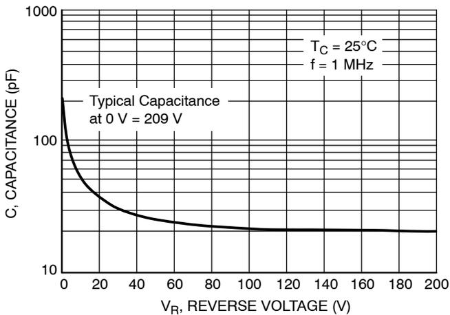
**Figure 5. Typical Capacitance**
