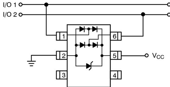
For this configuration, connect pin 5 directly to the positive supply rail ( $V_{CC}$ ), the data lines are referenced to the supply voltage. The internal TVS diode prevents overvoltage on the supply rail. Biasing of the steering diodes reduces their capacitance.
