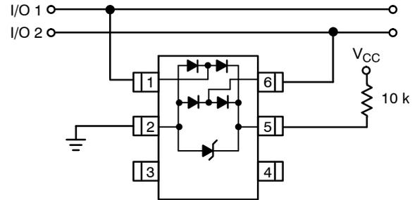
The NUP2202W1 can be isolated from the power supply by connecting a series resistor between pin 5 and  $V_{CC}$ . A 10 kΩ resistor is recommended for this application. This will maintain bias on the internal TVS and steering diodes, reducing their capacitance.
