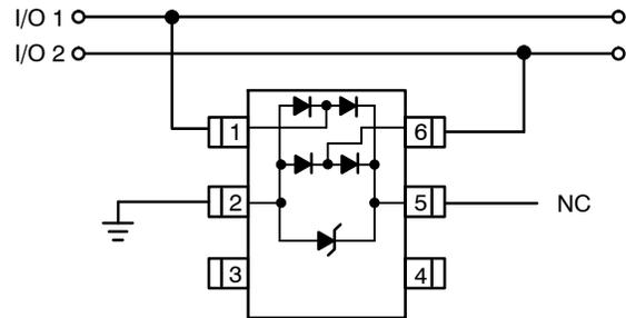
In applications lacking a positive supply reference or those cases in which a fully isolated power supply is required, the internal TVS can be used as the reference. For these applications, pin 5 is not connected. In this configuration, the steering diodes will conduct whenever the voltage on the protected line exceeds the working voltage of the TVS plus one diode drop ( $V_c = V_f + V_{TVS}$ ).
