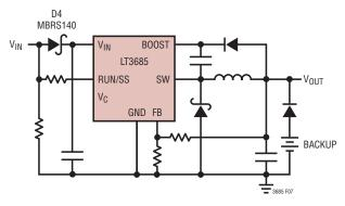
Figure 7. Diode D4 Prevents a Shorted Input from Discharging a Backup Battery Tied to the Output. It Also Protects the Circuit from a Reversed Input. The LT3685 Runs Only When the Input is Present
