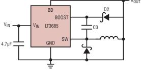
(4b) For  $2.5V < V_{OUT} < 2.8V$
