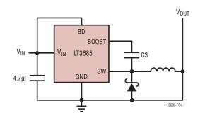
(4c) For  $V_{OUT} < 2.5V$ ;  $V_{IN(MAX)} = 30V$
