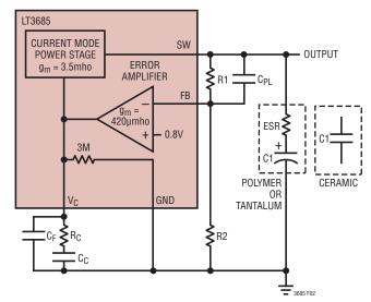
Figure 2. Model for Loop Response
