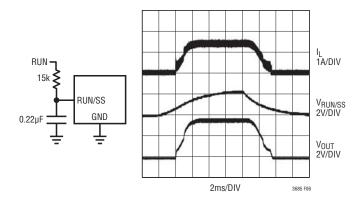
Figure 6. To Soft-Start the LT3685, Add a Resisitor and Capacitor to the RUN/SS Pin
