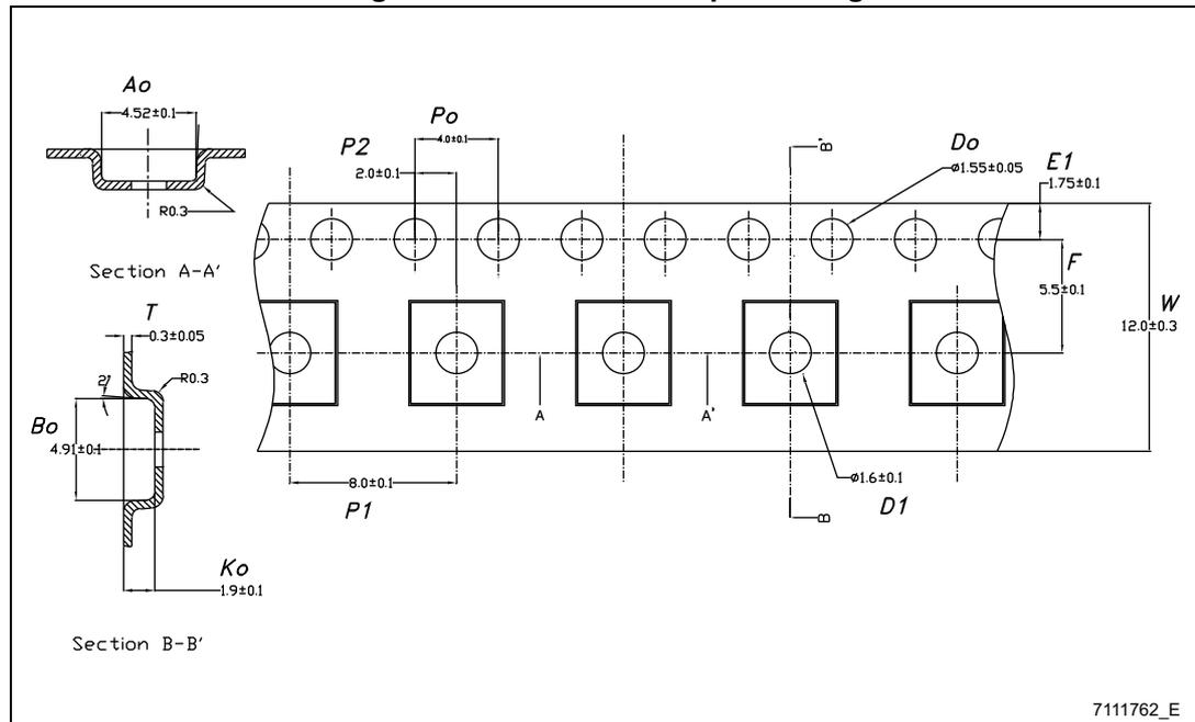
Figure 6. SOT-89 package orientation in carrier tape
